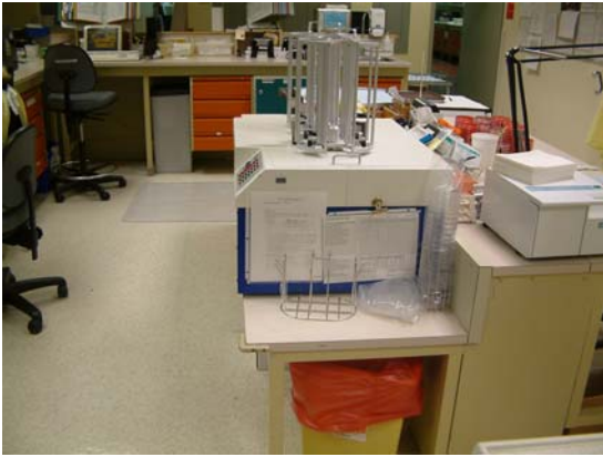
The height of the bench was adjusted, to lower the working height of the plate streaking machine
