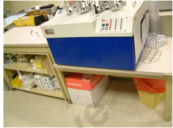
The height of the bench was adjusted, to lower the working height of the plate streaking machine
