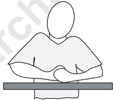
Awkward shoulder posture often results when the work surface is too high.
