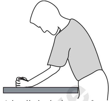
Awkward back and neck postures often result when the work surface is too low.
